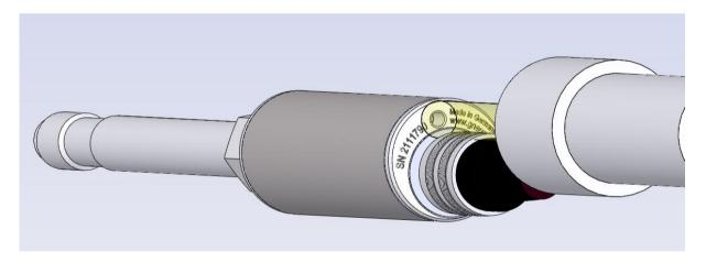
Insert the screw plug again afterwards; it simply serves for protection against contamination and extraneous light. The protection class is not impaired even without the screw plug being fitted. The integrated amplifier will thereafter transmit the starting value of its output scale (0V at 0...10V, 0mA at 0...20mA and 4mA at 4...20mA output signal. Function is suppressed, if the output signal is more than 5% of the maximum value.
